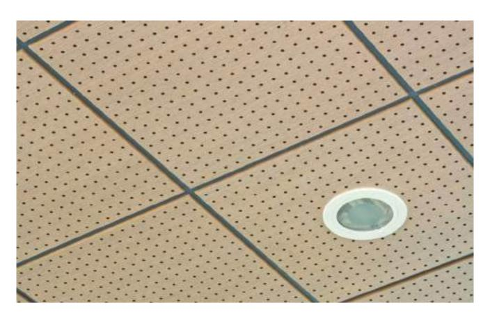
The Tacer Wooden lay in System is created with T-15 and custom-section carrier systems, and can be produced in standard 600x600 mm tile sizes or custom dimensions. These suspended systems are adjustable according to the client's preference for the drop height and can offer customized solutions. Tacer wooden panels are perforated and can be produced with adjustable hole density when acoustic performance is required.
